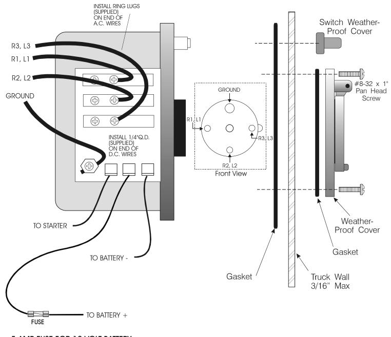
5 AMP FUSE FOR 12 VOLT BATTERY 3 AMP FUSE FOR 24 VOLT BATTERY IMPORTANT A FUSE MUST BE INSTALLED OR YOU WILL VOID THE WARRANTY.
